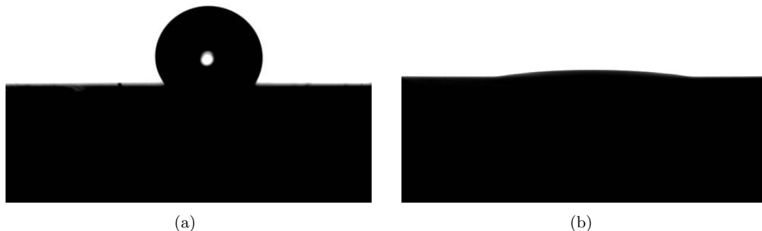
Figure 5.1: Images of drops taken during CA measurements (a) CA \sim 107^\circ , (b) CA \sim 8^\circ . Since these images, taken by the CCD camera of the CA goniometer, were actually used by the software to determine the CA, the contrast is very high so that only the shape is visible and the drops are not distinguishable from the surface material.
